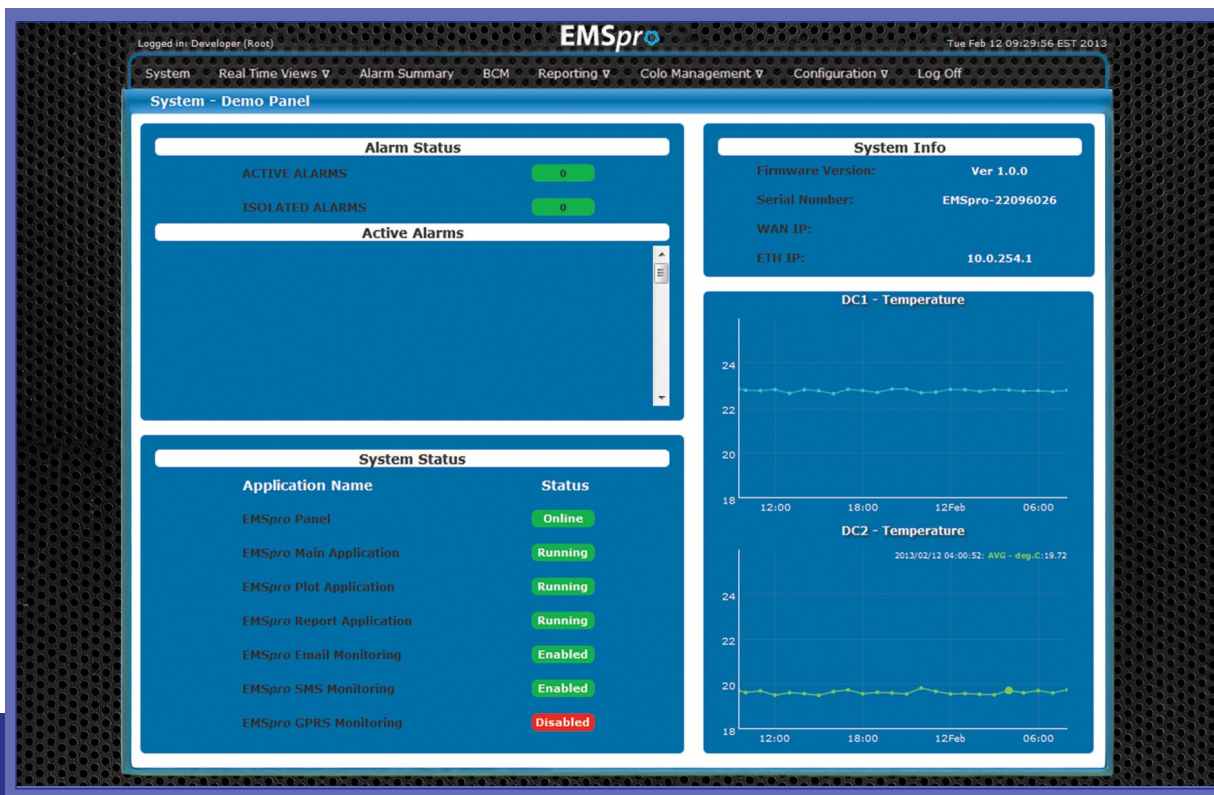
Diagram 2. System status page for an initial overview of the data centre including active and isolated alarms and general system status.
