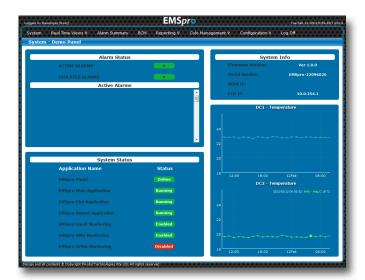
System status page for an in initial overview of the data centre including active and isolated alarms and general system status
